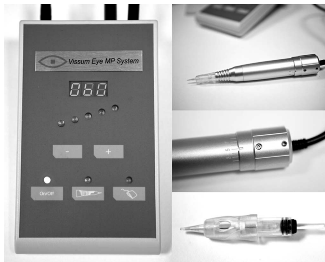
FIGURE 1. Superficial automated keratopigmentation device Vissum Eye MP system, Madrid, Spain (Apl. No. 2.949.539), provided by Blue Green Medical, Spain. (Left) The body of the device to which a handpiece is attached (right top). The distal part of the handpiece has a trundle (right center) that regulates the penetration depth of the needles. (Right bottom) Disposable tip that contains different numbers of needles depending on the area that will be pigmented.
